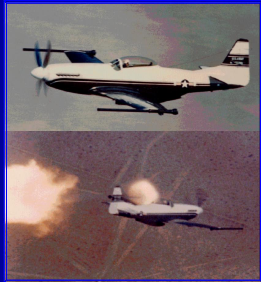
U.S. P-51 with 106 mm Recoilless Rifle on each wingtip
