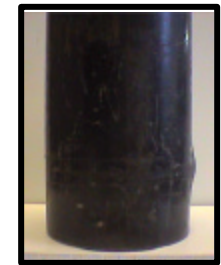
No Penetration Opposite Entrance Point
