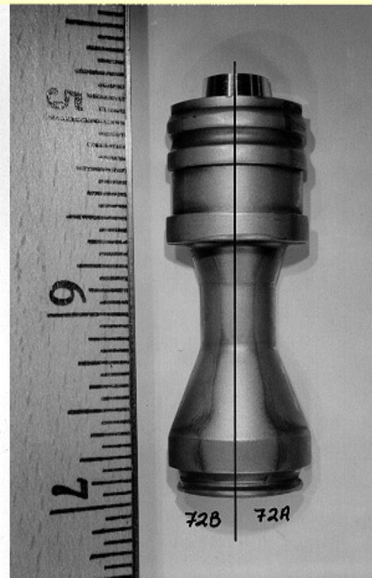
Figure 1b. Sabot No. 72 in the "as-received" condition, outer surface.
