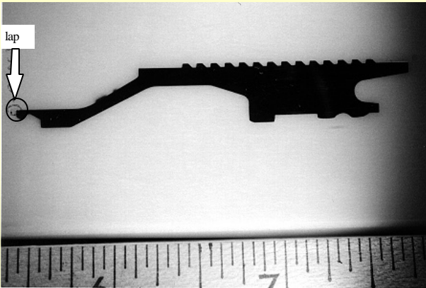
Figure 2a. Cross-section of Sabot No. 72A inside. The circled area is a lap that corresponds to Figure 2b.
