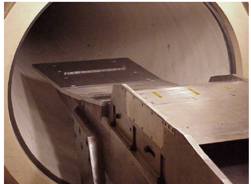
Full-Scale, H2 Scramjet Test – Feb 02 (Mach = 10)
