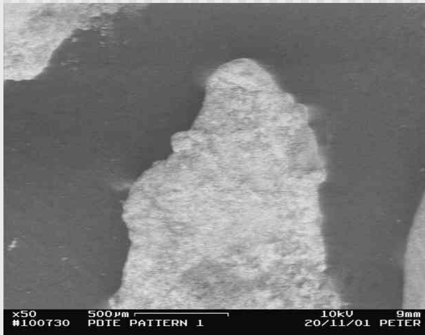
Enlarged Lead particle reveals cerussite
