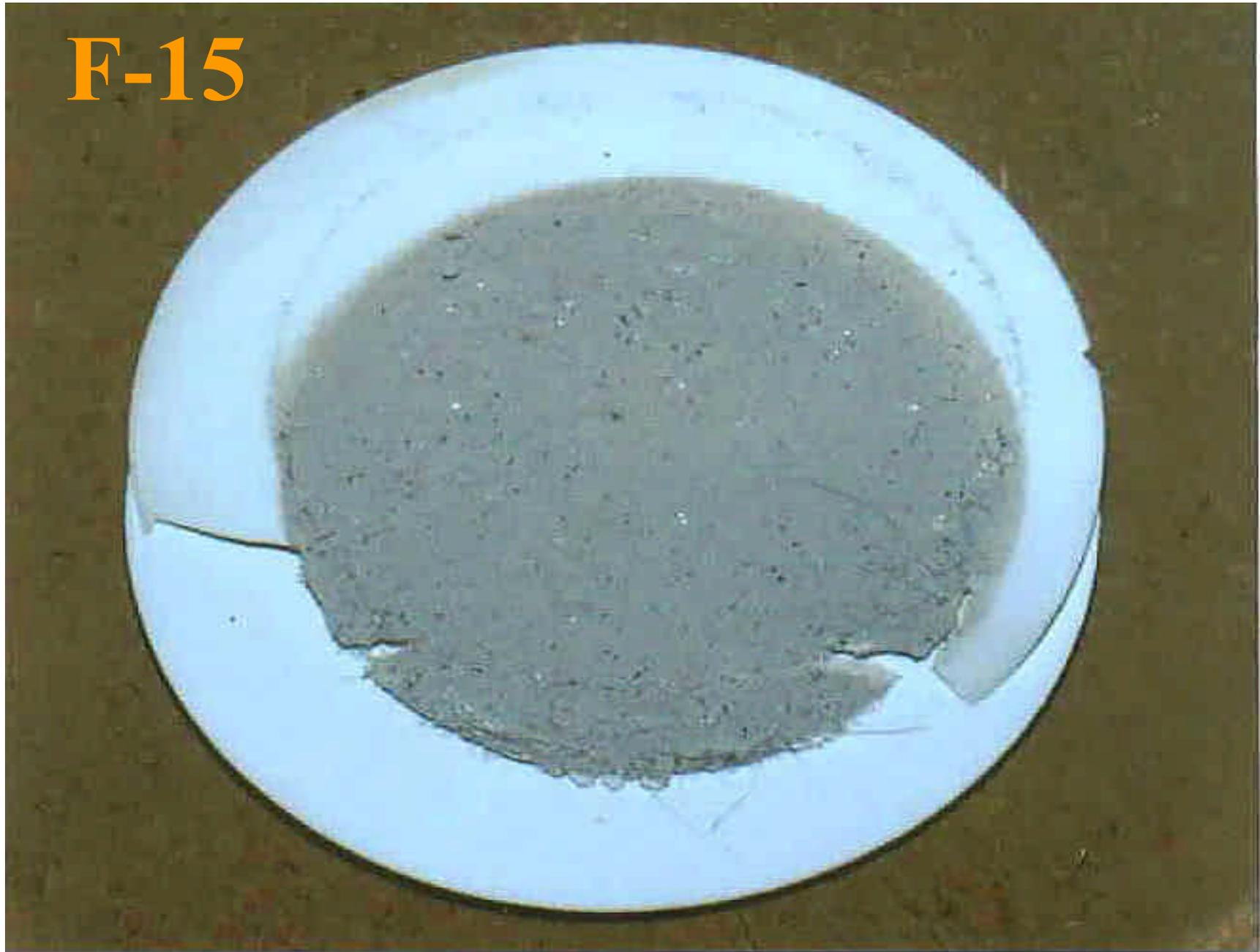
**Filter membrane with fine gray Teflon particles, traces of metal and paint chips extracted from felt.**
