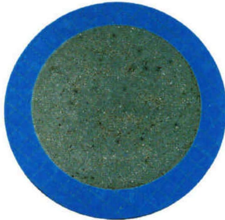
**Blue filter membrane with fine gray Al-Silicate particles extracted from felt.**
