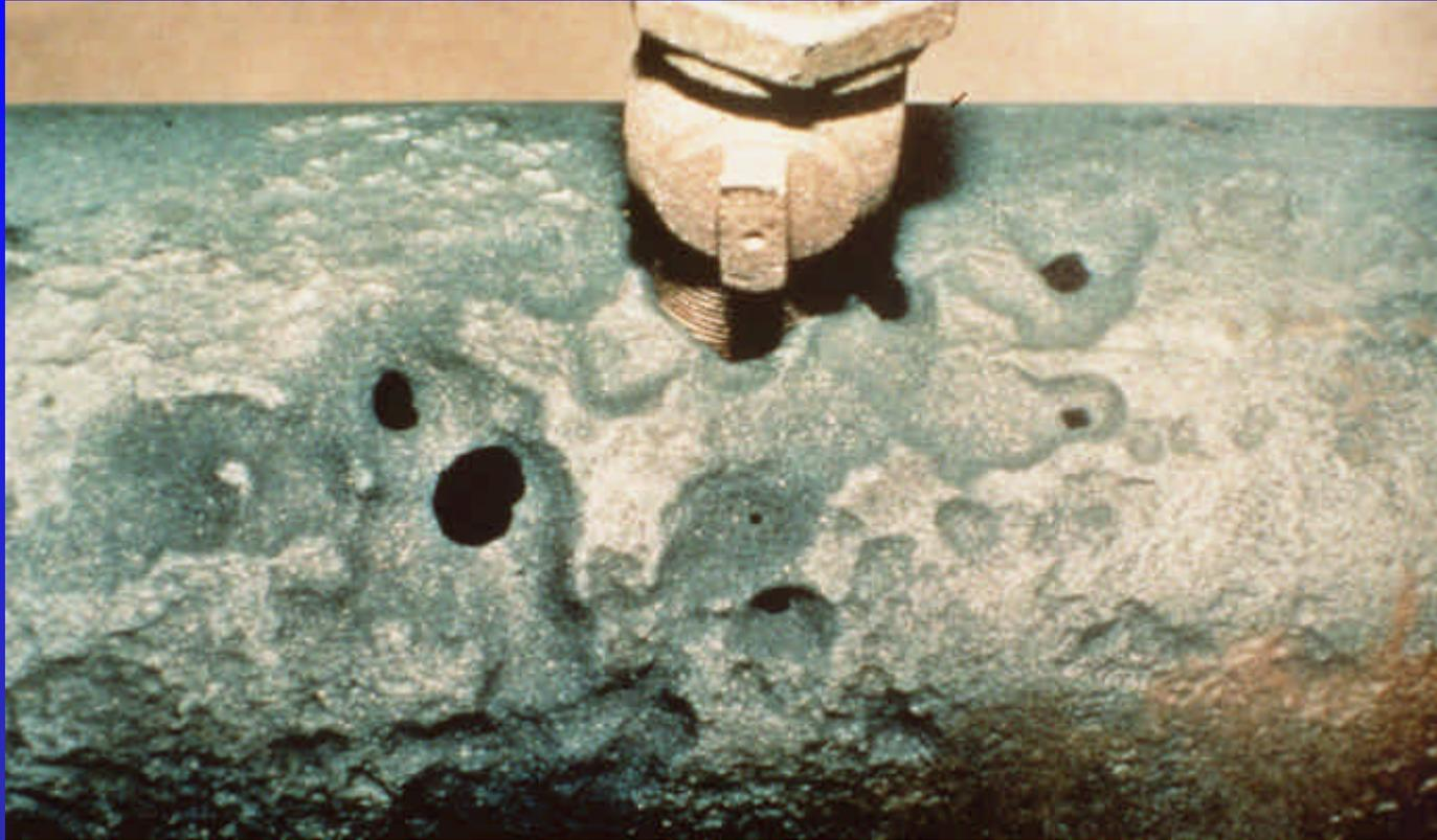
Corrosion of iron when coupled to copper service line.
