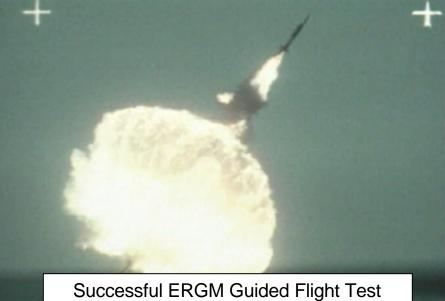
Successful ERGM Guided Flight Test 4m accuracy
