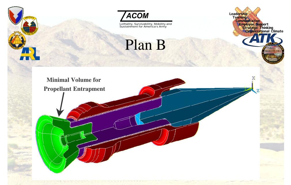
Eliminate Trapped Propellant by Pushing the Tail Cone Forward
