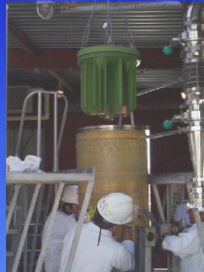
Positioning pulse 1 mandrel
