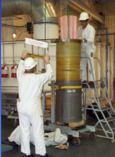
Installing pulse 2 mandrel in case
