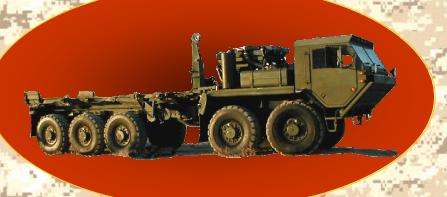
The LVSR will replace the current heavy tactical vehicle fleet system that transports bulk liquids (fuel/water), bulk and break bulk cargo, standardized containers, ammunition and bridging. The LVSR will provide a 5th wheel capability to haul heavy combat/engineer equipment and will provide the Marine Corps' heavy wrecker/recovery capability.
