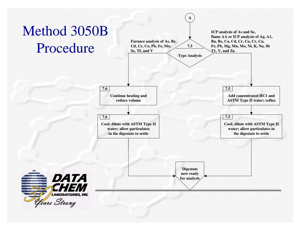
NOTE: Section 7.5 may be used to improve the solubilities and recoveries of antimony, barium, lead, and silver when necessary. These steps are optional and are not required on a routine basis.
