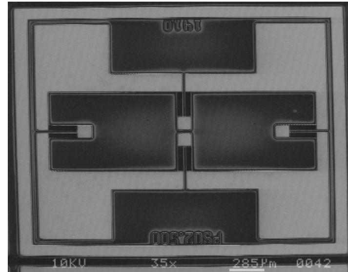
3. SEM micrograph of Gen 2 NASA sensor (with boss)
