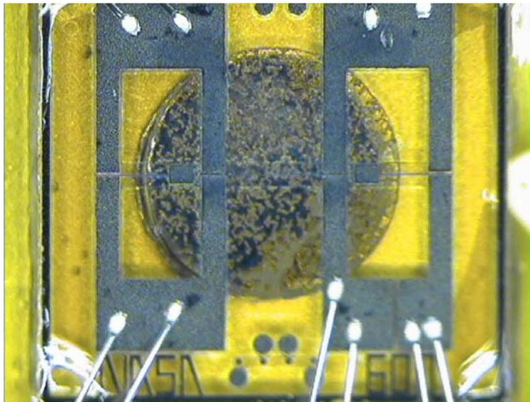
2. Optical micrograph of Gen 1 NASA sensor (no boss)
