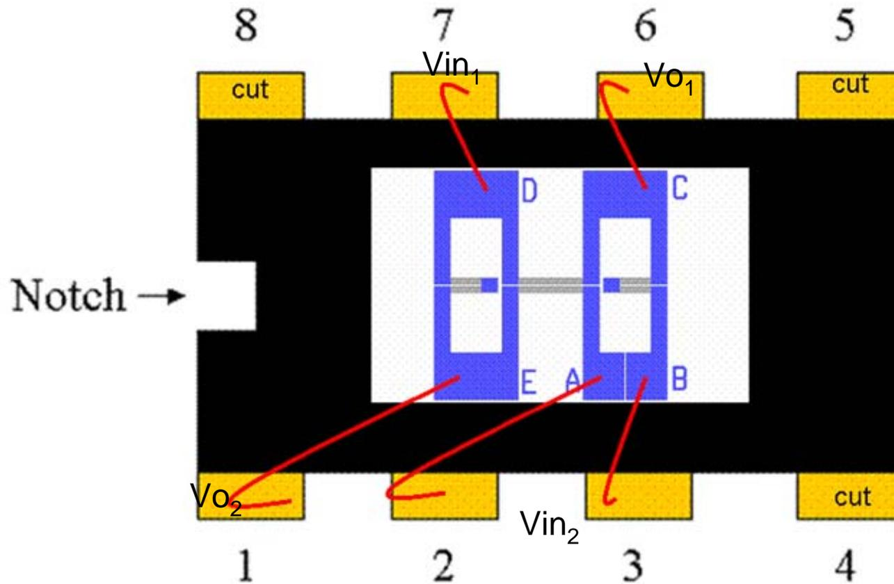
The above configuration makes the Wheatstone Bridge an open one. It allows each resistor element BC, CD, DE, and EA to be measured independently. When 2/3 is connected together, the bridge is closed. To be consistent, the power supply  $V_{in_1}$  and  $V_{in_2}$  should be connected at pin 7 and 2/3, respectively. The output  $V_{o_1}$  and  $V_{o_2}$  should be tapped at pin 6 and 1, respectively.
