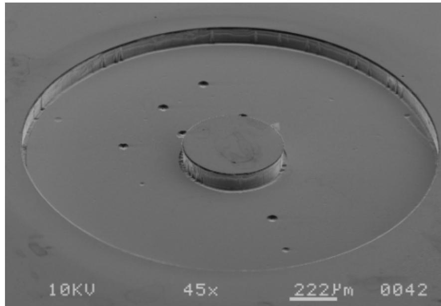
**A SEM micrograph of the backside deep reactive ion etch for the NASA bossed sensor.**
