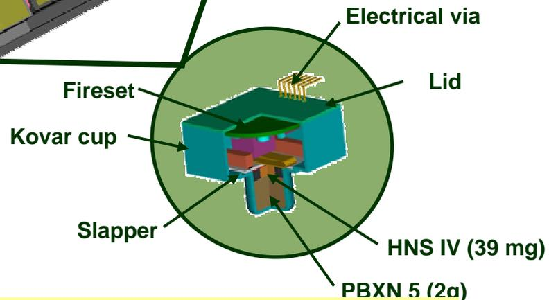
• **Integrated high voltage Initiator package (Fire-set, Slapper, Leads)**
