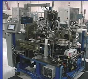
QSI Slide Sub-Assembly Molding Machine
