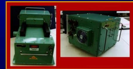
Electro-Optical Test Set (EOTS)
