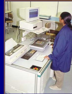
**In-Circuit Testing (Teradyne)**
