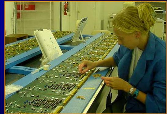
**Thru-Hole PWB Assembly**
