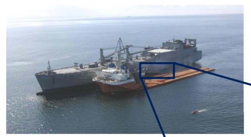
LMSR USNS Watkins and FLO/FLO Ship MS1 rafted and underway in calm water. The Watkins sideport ramp is down on the MS1 and ready for vehicle operations.
