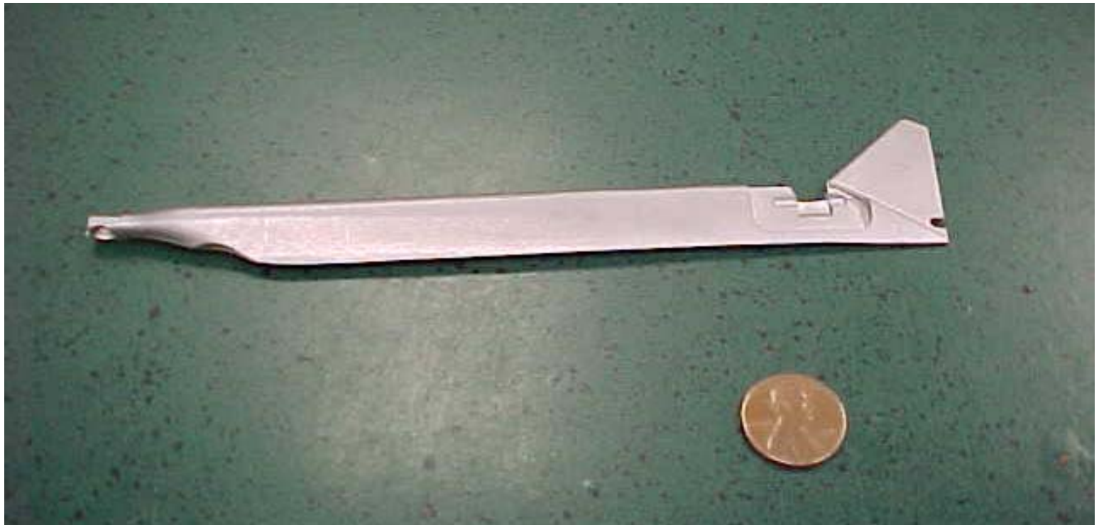
As-sintered 17-4PH Flaperon
