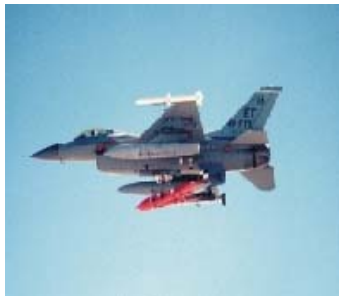
Joint Air to Surface Strike Missile (JASSM) 2250 pounds, 14 Feet Long Big Platforms
