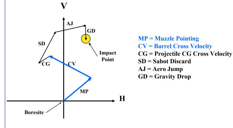
Objective: Make MP & CV small, repeatable on a barrel-barrel basis
