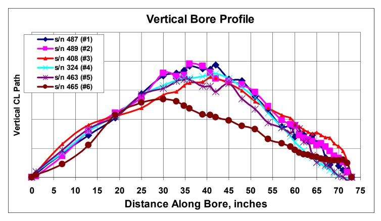
Barrels supported at aft & mid barrel (~ 39") Mathematically zeroed at breech & muzzle
