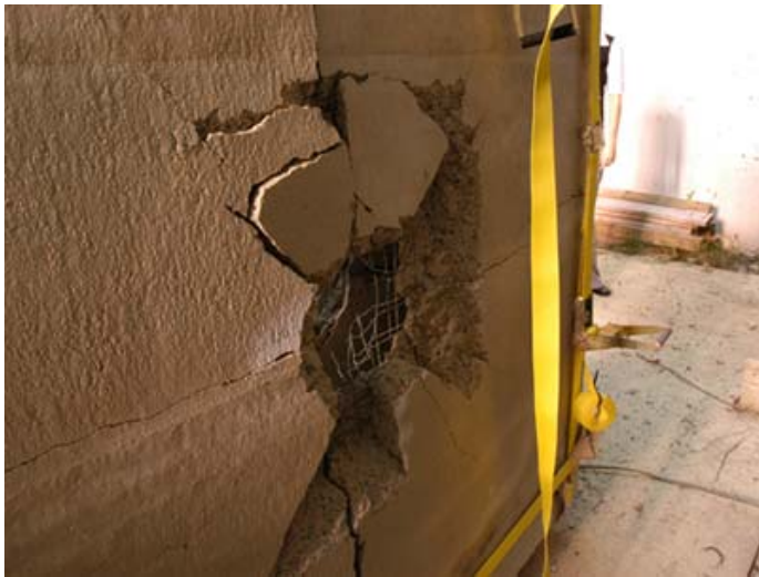
Entrance Hole, Test PGM-C01 10.5" 5K RC
