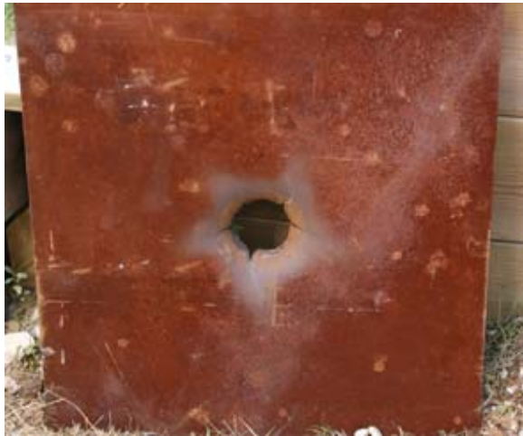
Penetration Hole in 0.5-in. RHA Steel
