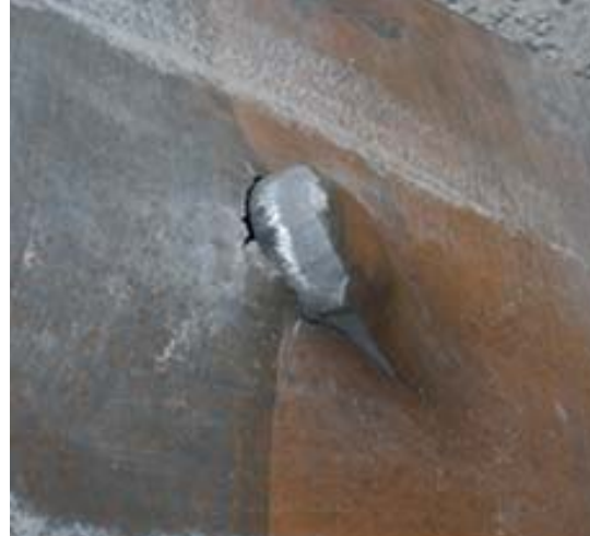
Bulge in 1-in. RHA Steel Plate, Exit View
