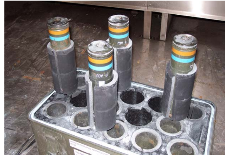
Some Deterioration of Packaging
