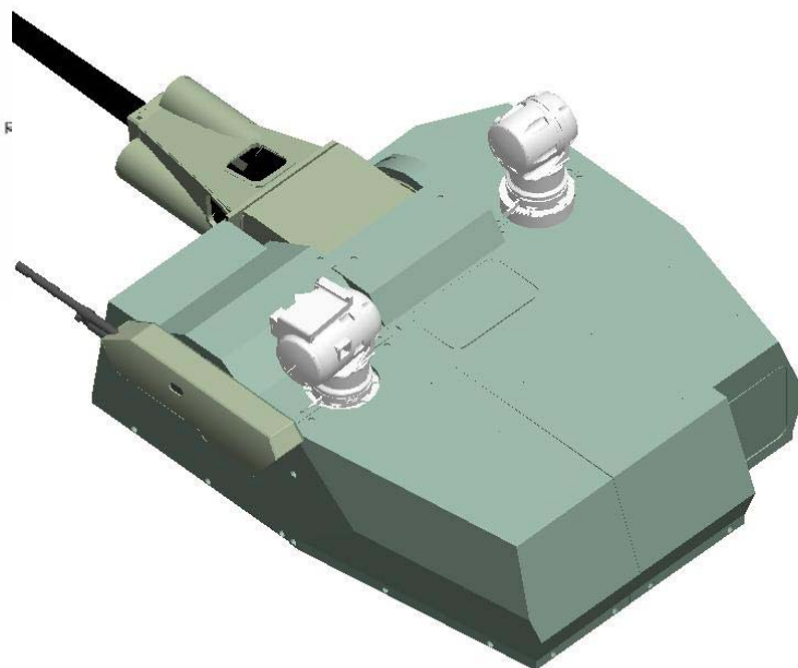
Unmanned Turret 1,5 tonnes Protection Level 3
