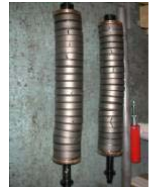
Recoil System Ring stack Failed in Fatigue
