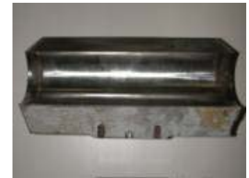
Chamber failed in fatigue
