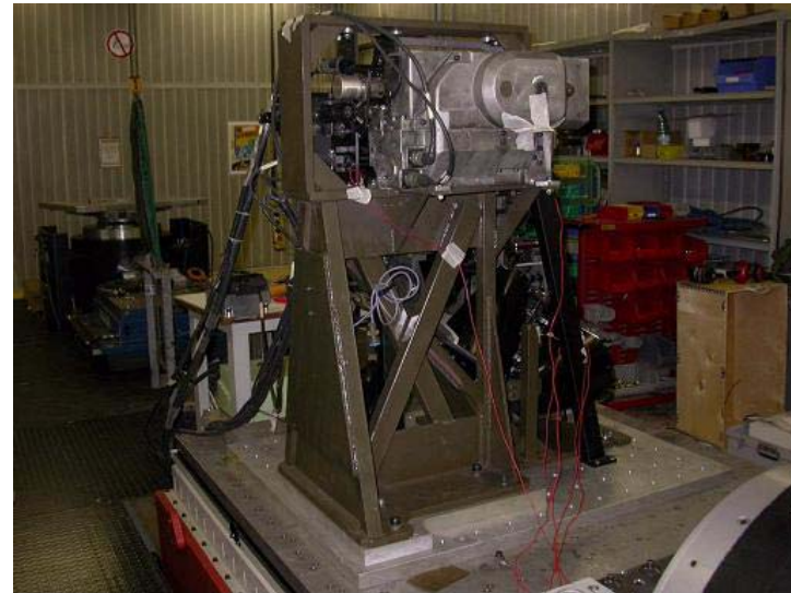
Feed System on Vibration Table November 2004
