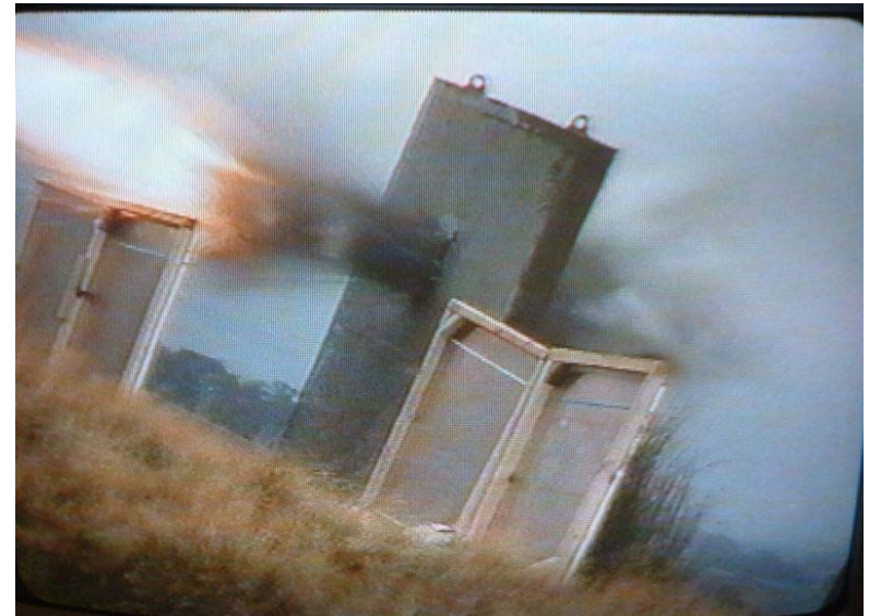
Defeat of Armoured Concrete with Behind Armour Effects
