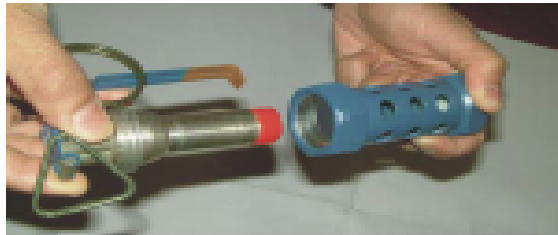
Figure 3-5b. Screwing the M240 Fuze Cartridge onto Grenade Body.
