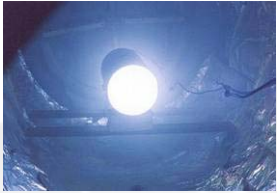
Hollow cathode discharge in hydrogen and argon for cleaning
