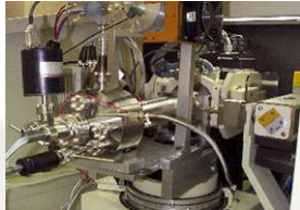
In-situ deposition for coatings diagnostics during growth
