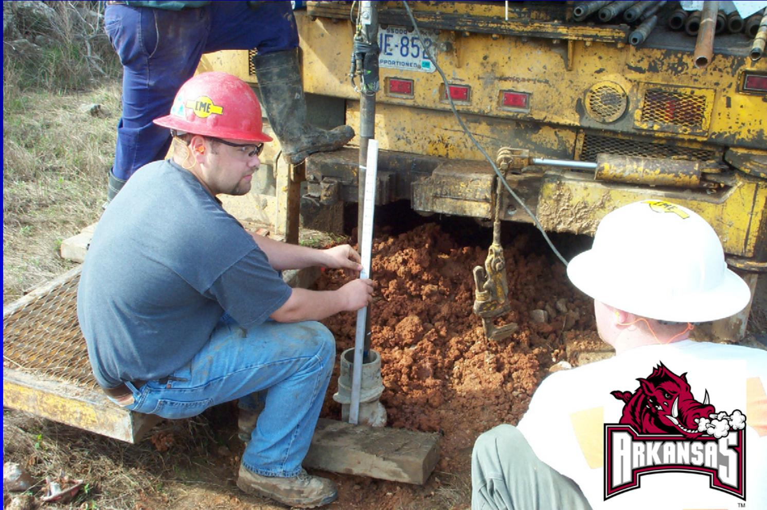
Instrumented Drill Rod to Measure Hammer Energy
