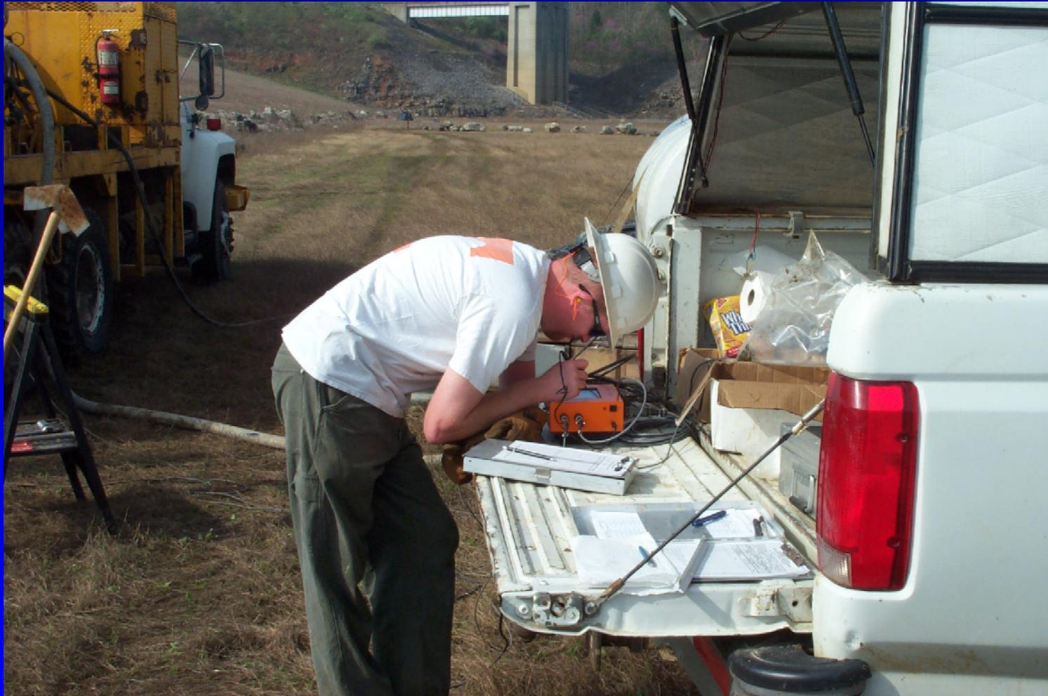
SPT Analyzer Readout Terminal
