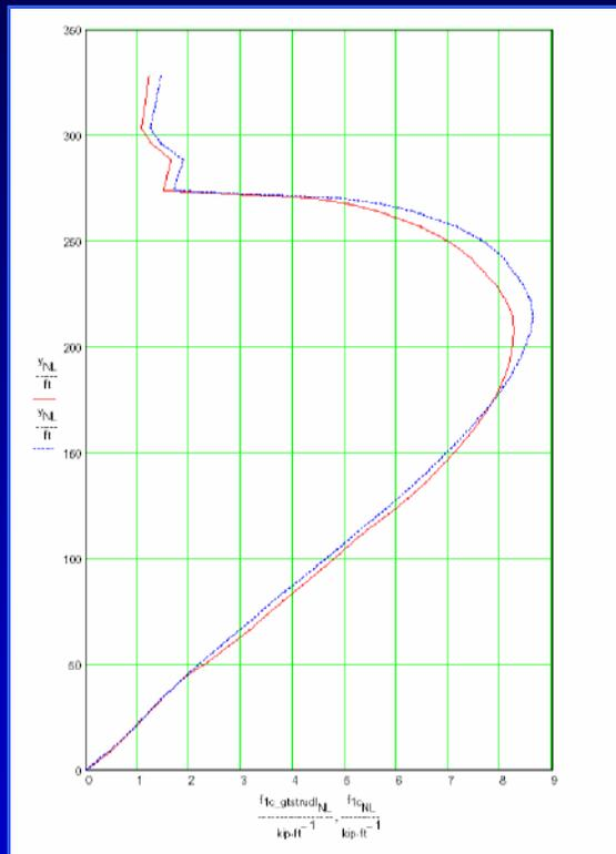
Inertia forces associated with fundamental mode response
