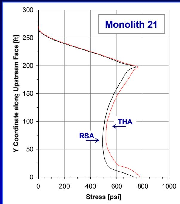
**RSA** → Maximum stress estimate obtained with the response spectrum approach considering horizontal and vertical input ground motion.
