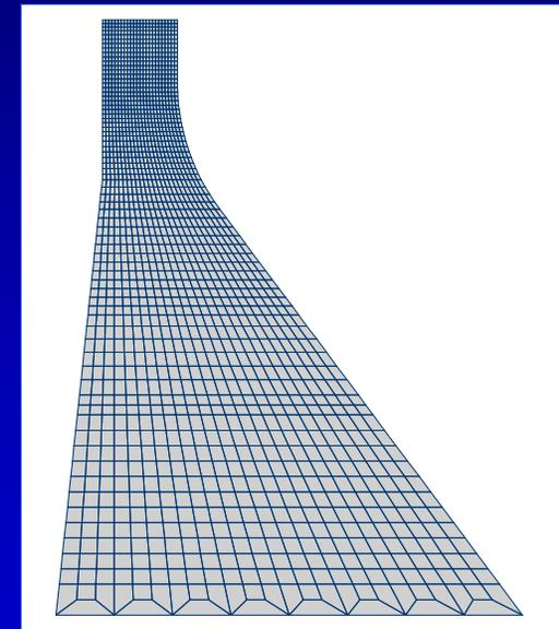
Finite-element mesh for non-overflow Monolith 21
