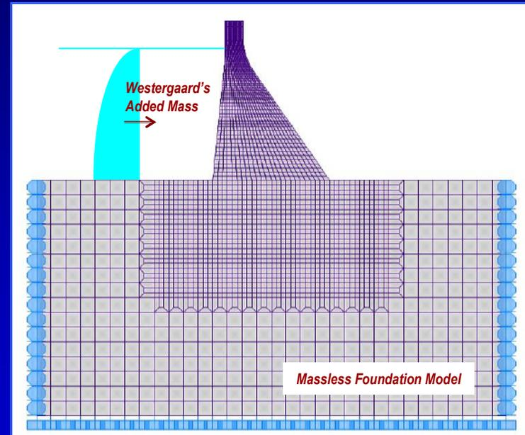
Finite-element mesh for
