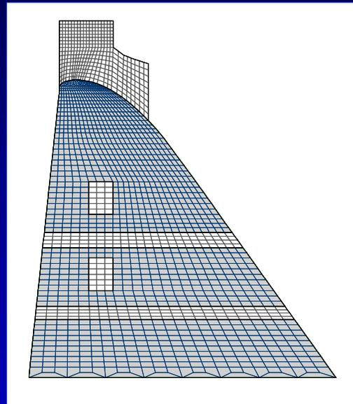
Finite-element mesh for spillway Monolith 14
