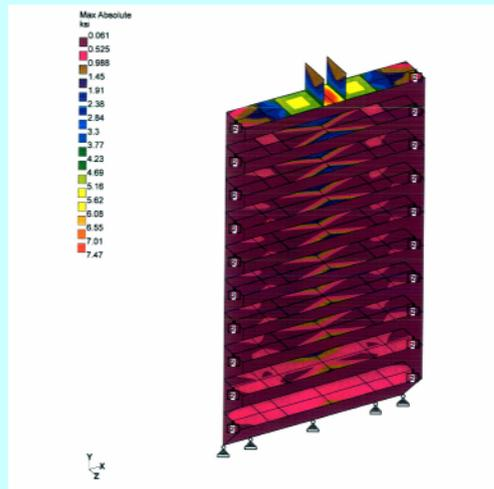
Figure-7 Stress Contour (Machinery load)
