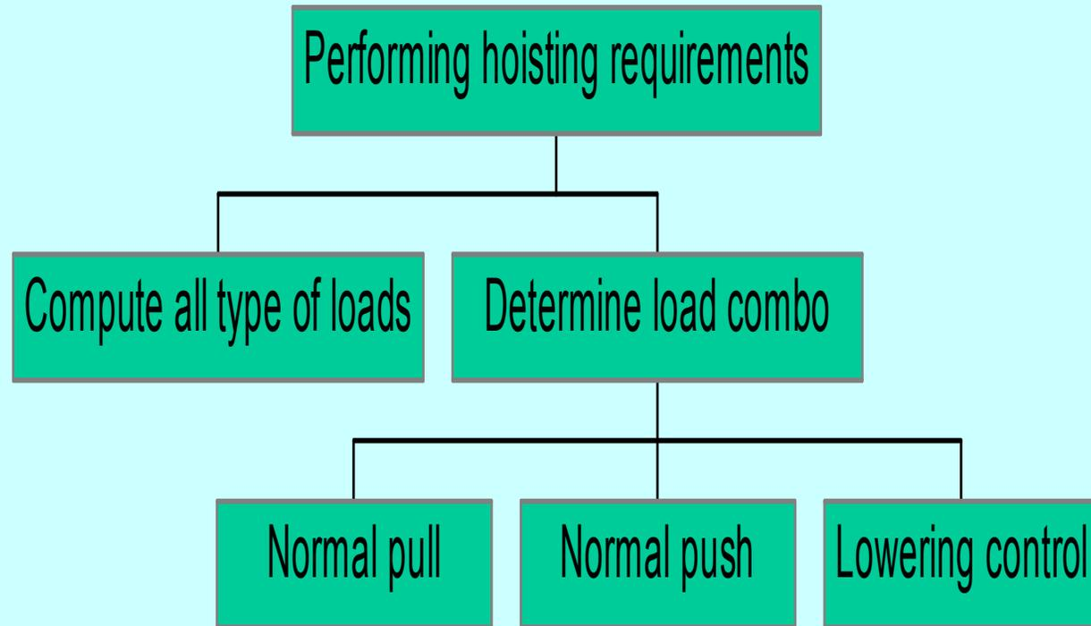
**NOTE:** Hoisting requirements are determined to estimate cylinder size and max. push requirements.
