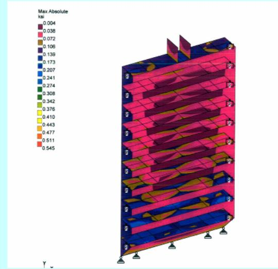
Figure-2 Stress contour (Self Weight)
