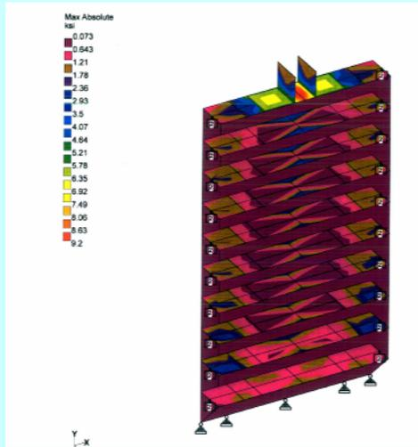
Figure-9 Stress Contour (Load combo-1)
