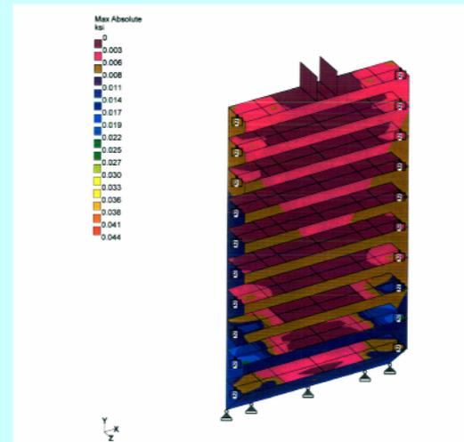
Figure-8 Stress Contour (Buoyancy load)
