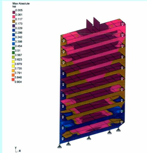
Figure-5 Stress Contour (Down pull load)
