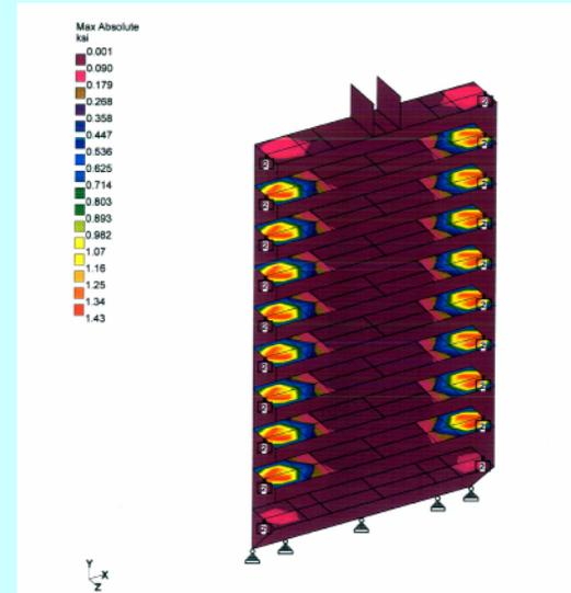
Figure-6 Stress Contour (Wheel load)
