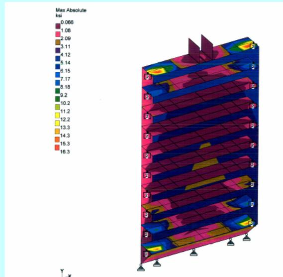
Figure-3 Stress contour (Hydrostatic load)
