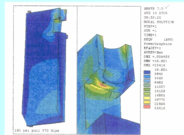
Figure-4: Gate slot cut-out close-up view (ANSYS)
