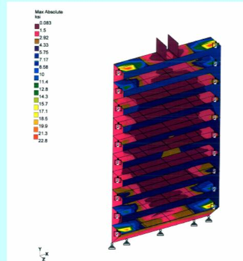
Figure-10 Stress Contour (Load combo-2)
