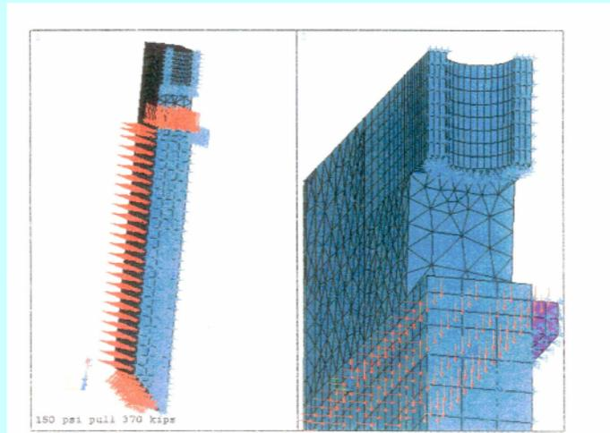
Figure-1 Slide Gate ANSYS mesh generation
