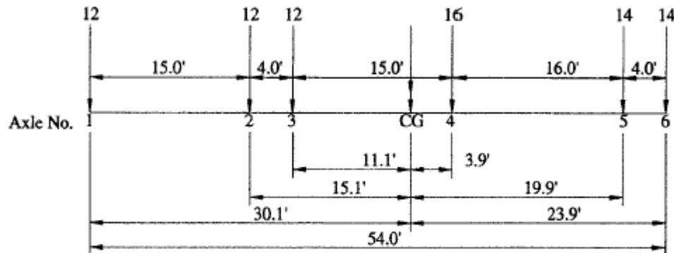
Figure B.6-4 Type 3-3 Unit WEIGHT = 80 kips (40 tons).
