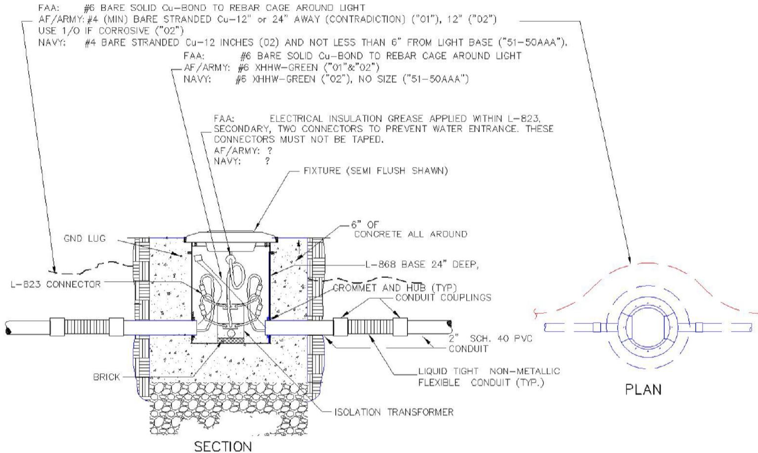
L-868 BASE DEEP CAN METHOD (GREEN GROUNDING CONDUCTOR—SEPARATE COUNTERPOISE)
