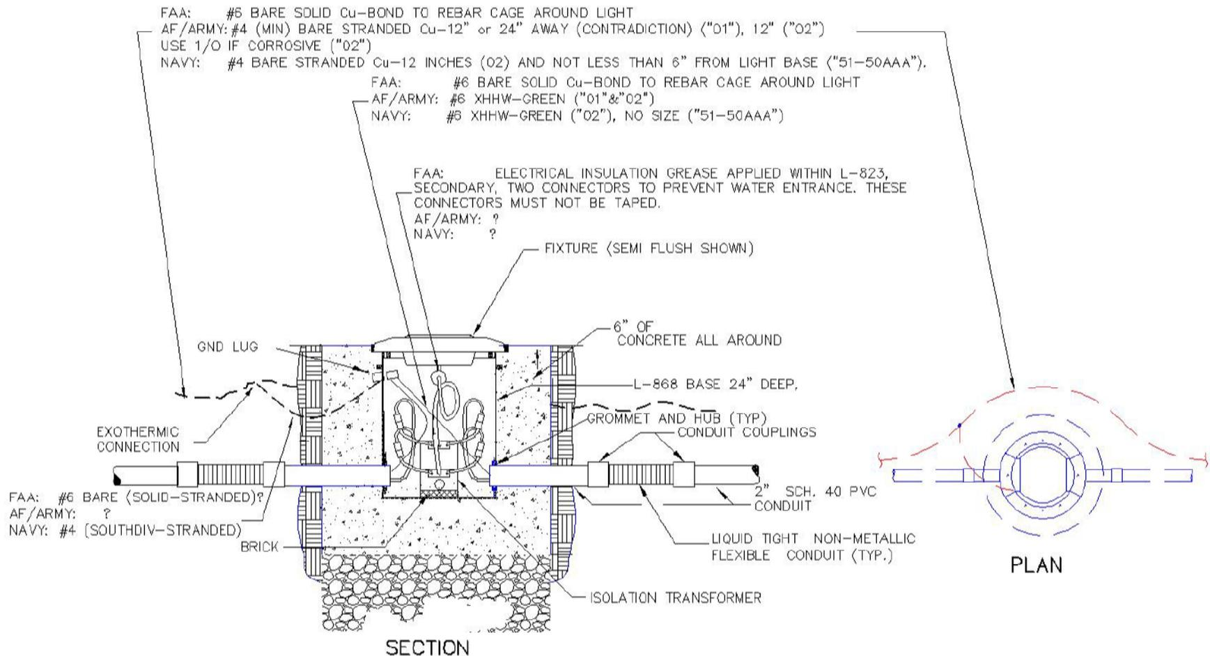
L-868 BASE DEEP CAN METHOD (GREEN GROUNDING CONDUCTOR CONNECTED TO COUNTERPOISE)
