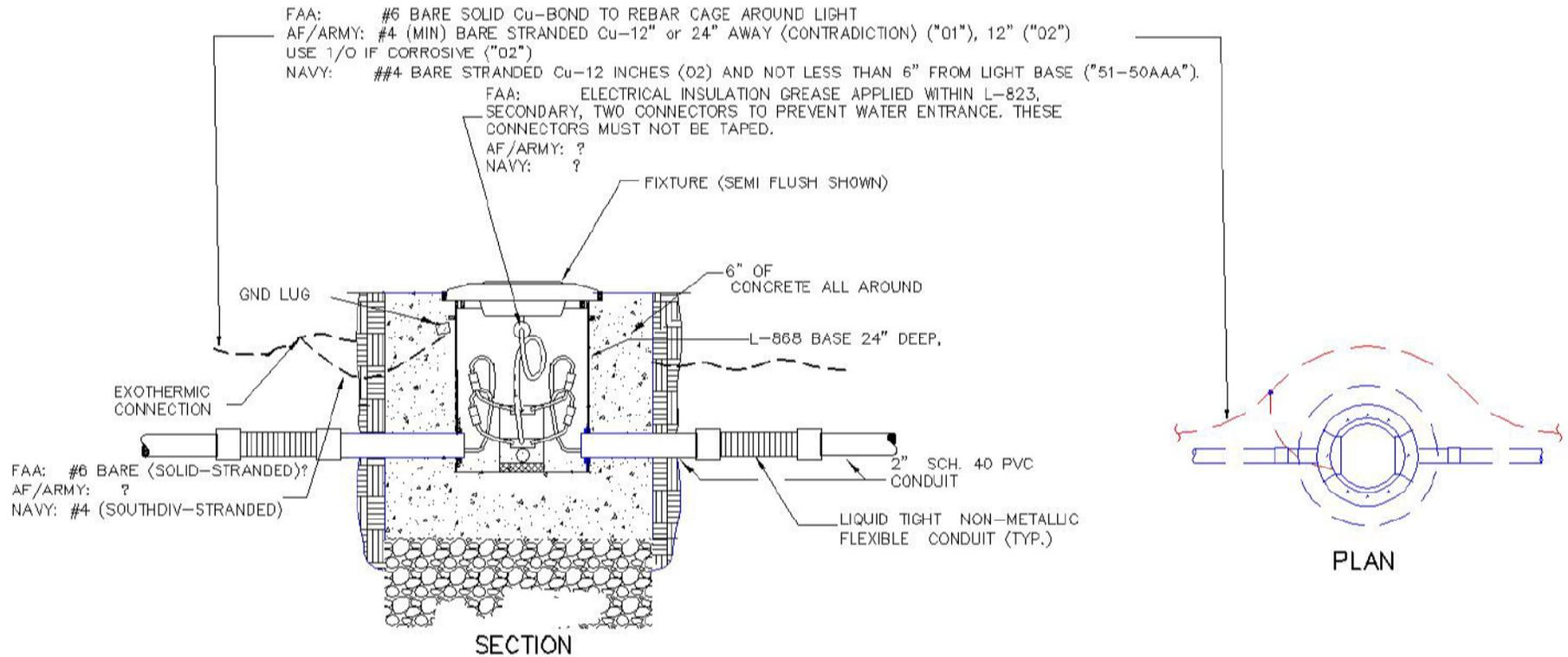
L-868 BASE DEEP CAN METHOD (BASE CONNECTED TO COUNTERPOISE)
