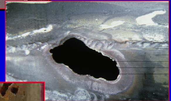
Boiler Tube – Oxygen Pitting Failure
