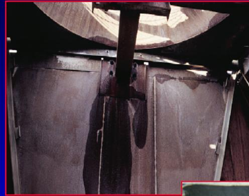
Poor control of acid feed strips galvanizing
