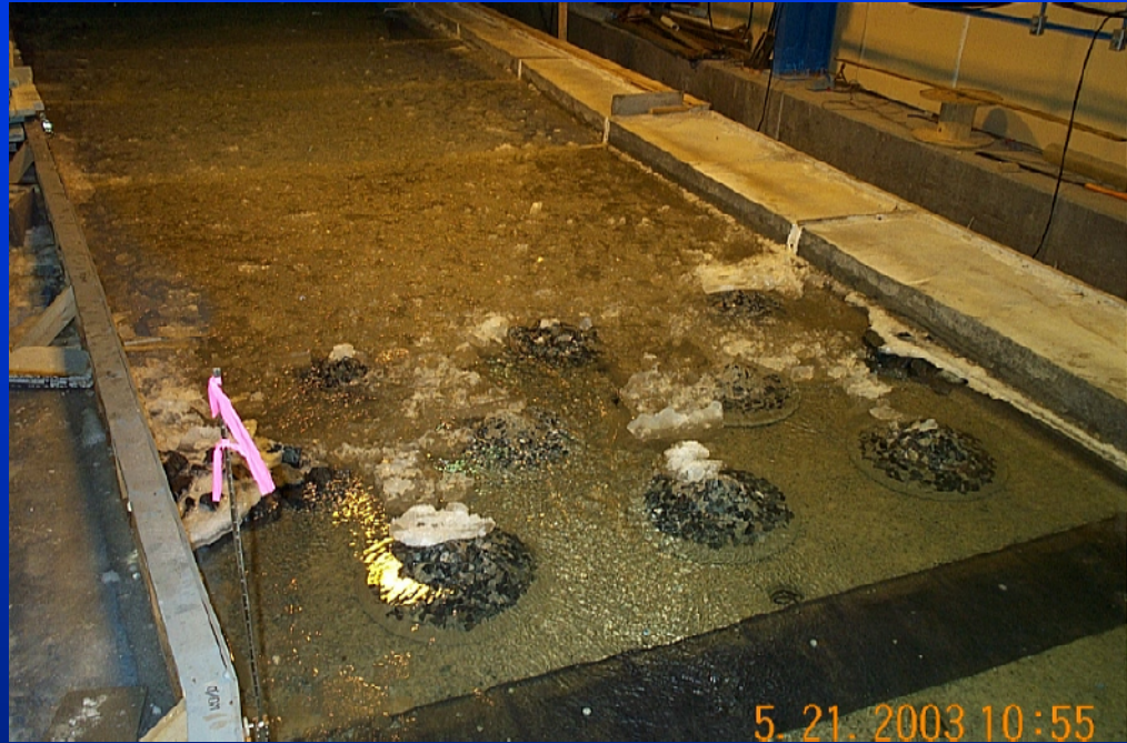
Array of artificial islands as a more aesthetic alternative to concrete piers. Performance similar to piers.
