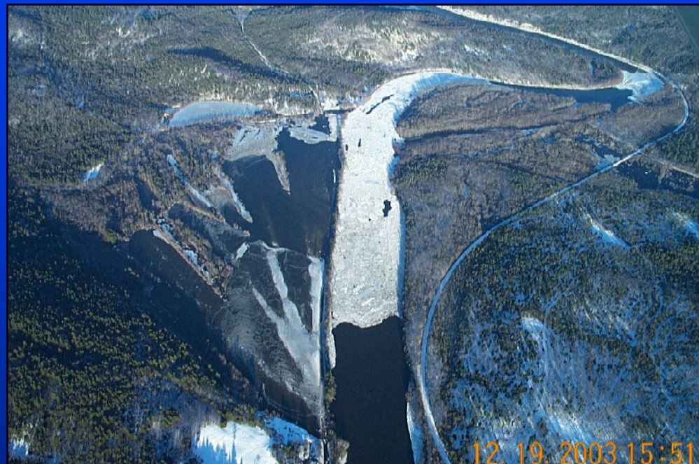
Ice jam in constricted bend in the Androscoggin River downstream of Canton, ME.
