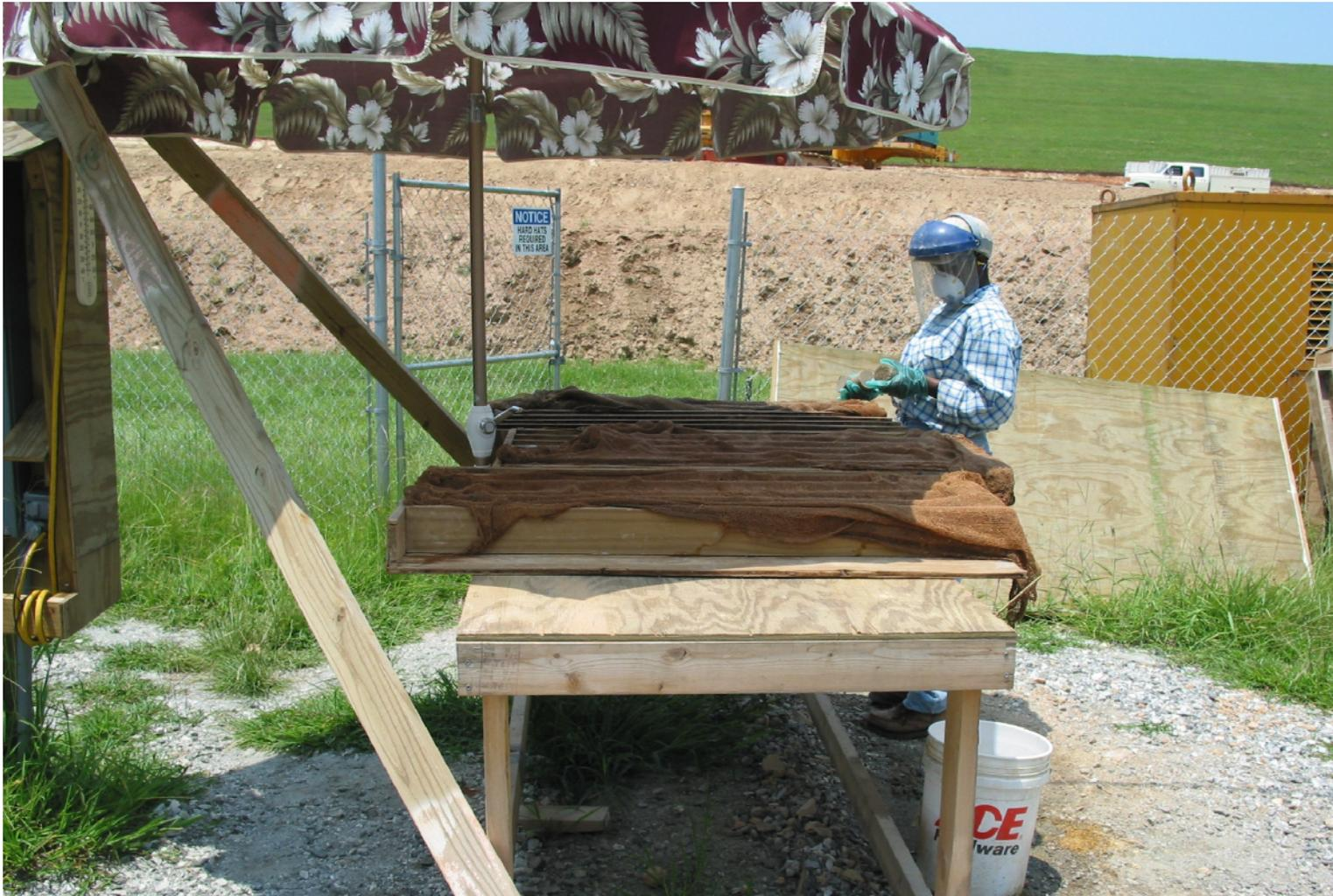
Logging of core and selecting test specimens
