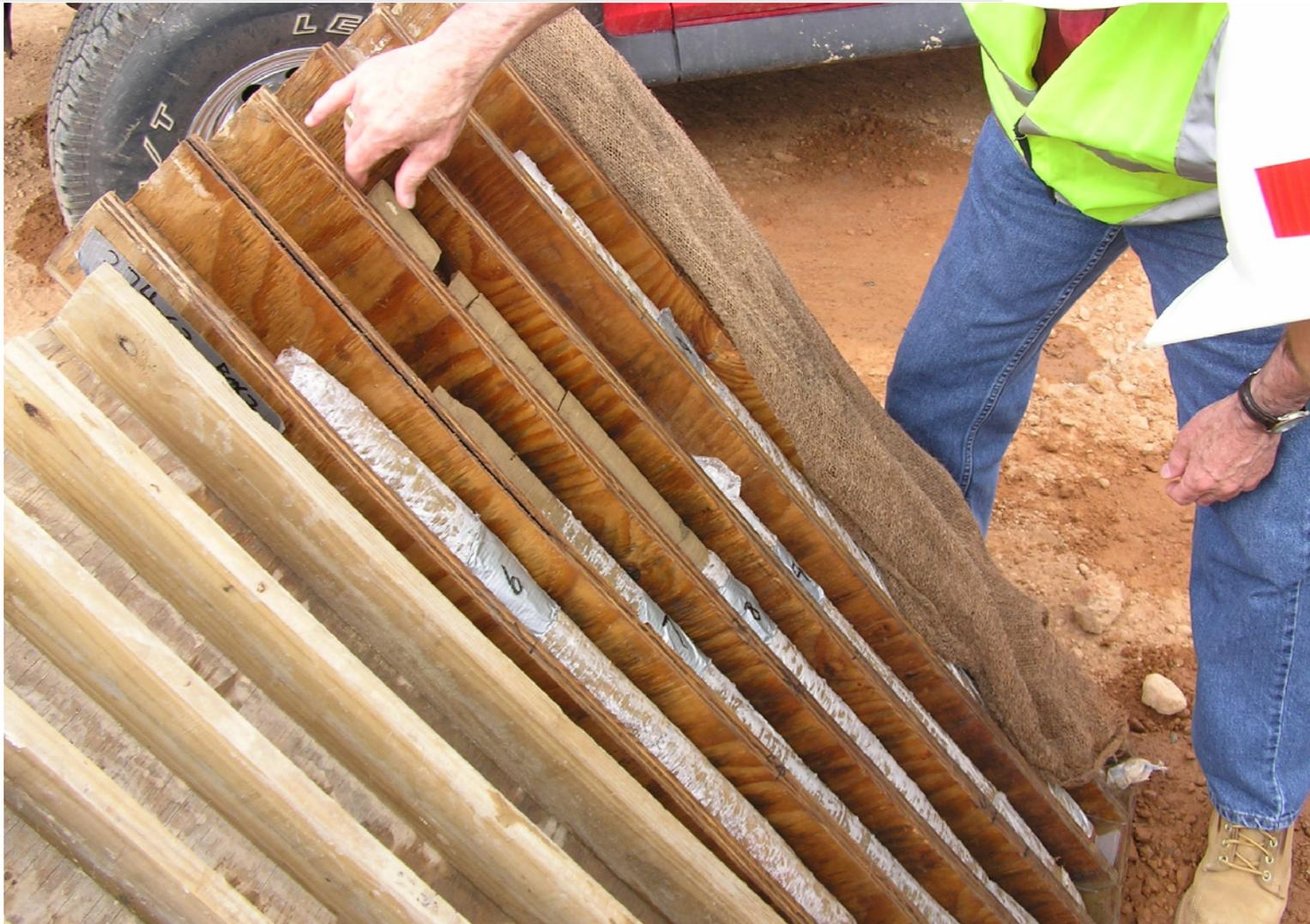
Core in core box; note plastic sheath and burlap
