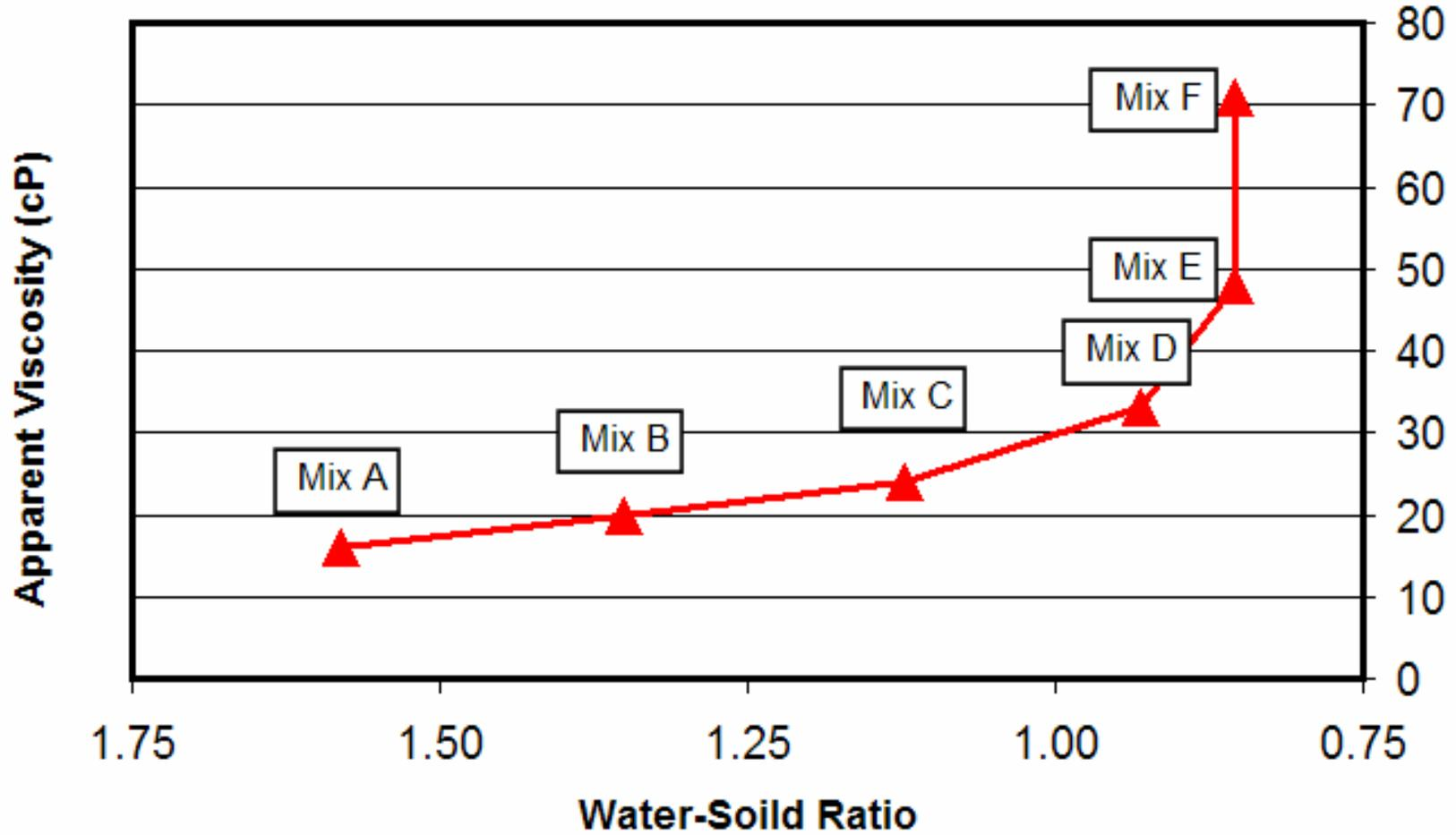
**Relationship of Apparent Viscosity and Water-Soild Ratio**
