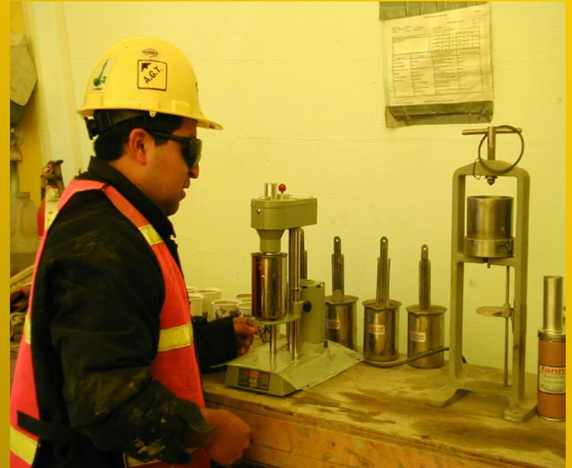
$$K_{pf} = \frac{\text{volume of water ejected}}{\text{initial volume of grout} \times (\text{filtration time (min)})^{1/2}}$$
