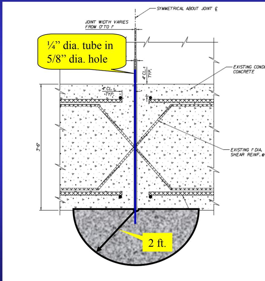
Assuming that grout is injected at the bottom of the conduit and expands radially from the injection point. For example if 2.7 gallons were injected at a hole, the radius of the hemisphere created would be 24.5 inches.
