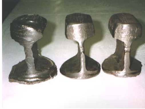
Buried steel railroad rails cored with Sonic
