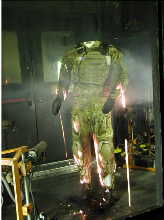
After-burn and melt drip on nylon at lower leg, around knee and elbow pads
