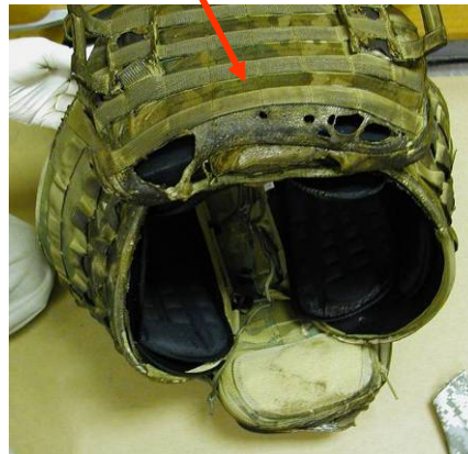
Interior of chassis was unaffected. Slight singeing lower edge of inner pads. 1,000 denier nylon on outside of chassis stayed mostly intact.
