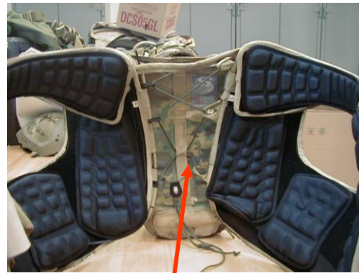
Interior of chassis was unaffected. Slight singeing lower edge of inner pads. 1,000 denier nylon on outside of chassis stayed mostly intact.
