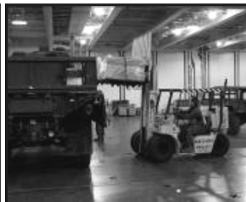
Pallets are placed in vehicles from one side or from the rear while keeping traffic lanes to other bays clear.
