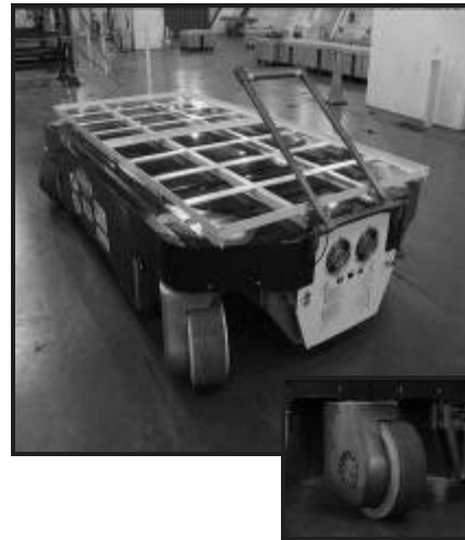
Compact Agile Material Mover (Camm), Oak Ridge National Lab, Operated by NSWC Philadelphia
