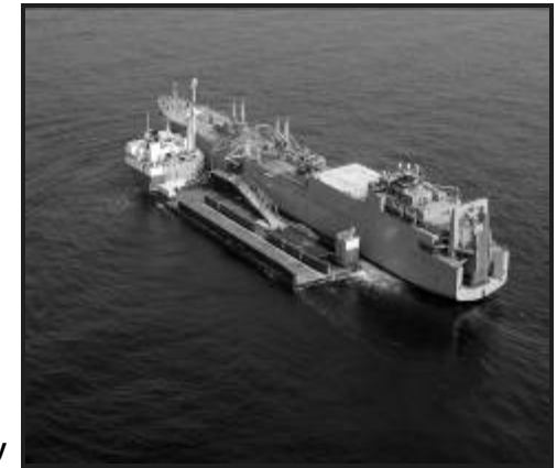
the ramp is lifted along the guideposts and deployed to the deck of the Mighty Servant 3.
