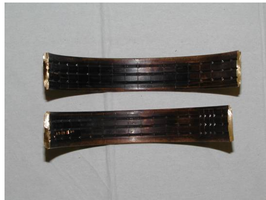
Swaged Copper alloy rotating band
