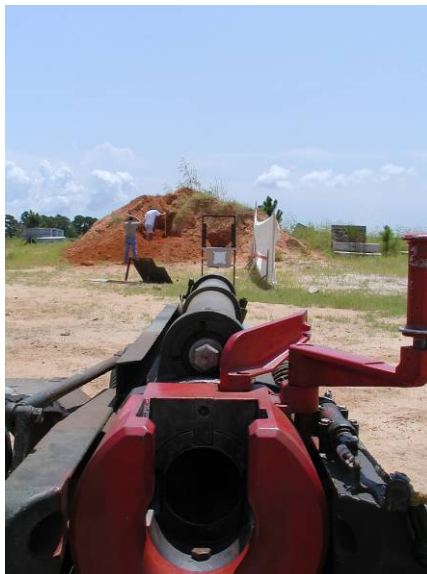
Sand target for soft recovery
