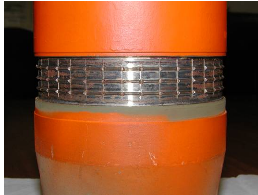
Swaged Copper alloy rotating band
