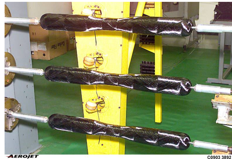
Multiple spindles increase production rate
