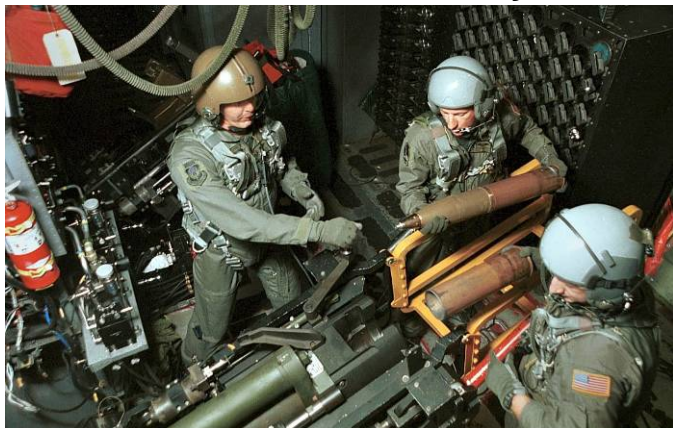
Aircrew loading 105mm round into M102 Gun System derived from the Army field artillery M1A1 howitzer
