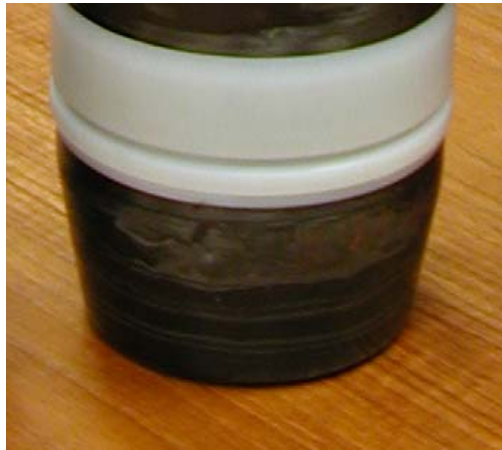
Boat tail machined from composite body
