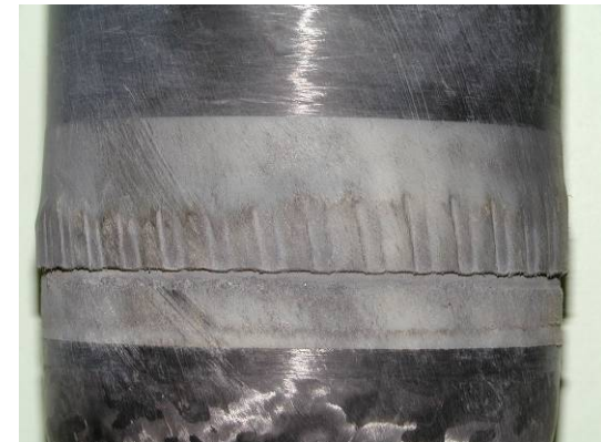
Post launch rotating band intact
