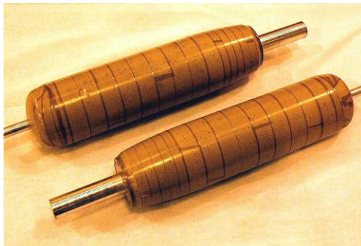
Sand mandrel overlaid with non-stick tape
