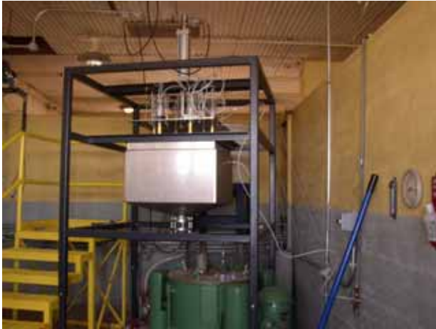
Sonication tank positioned above centrifuge.
