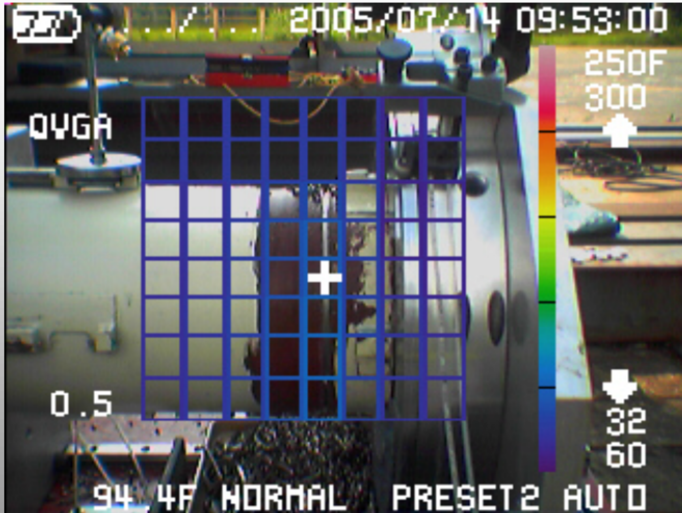
Thermal Image of Cut
