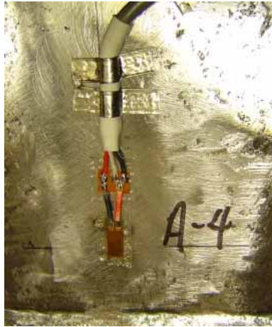
Strain gage installation
