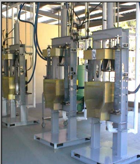
Warhead Billet Splitting Machines
