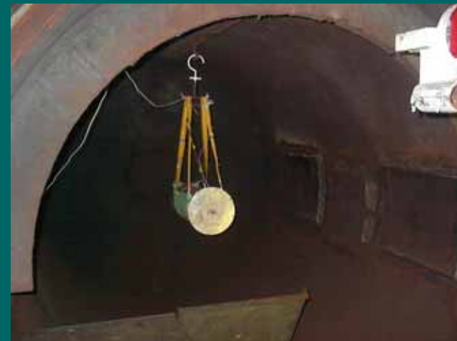
Simulated bomb with donor charge hung in DAVINCH chamber
