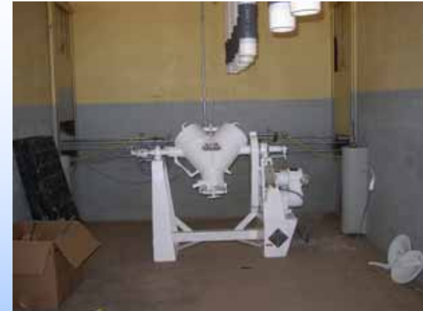
Vacuum cone dryer in bay 6B
