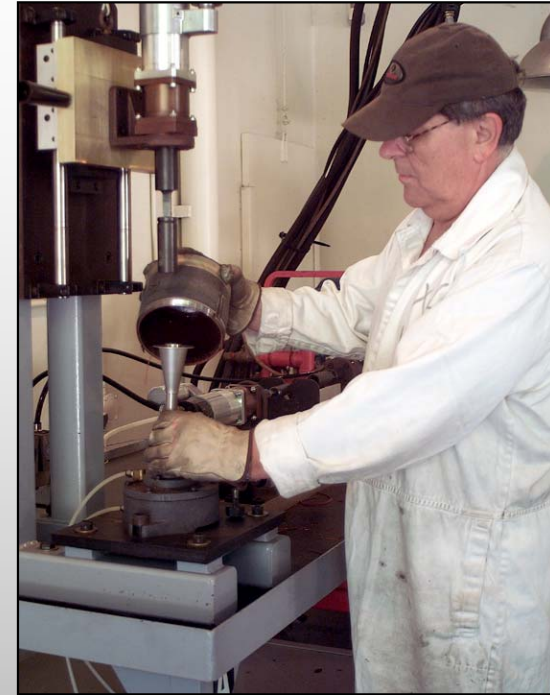
TOW Igniter Assembly Removal Machine
