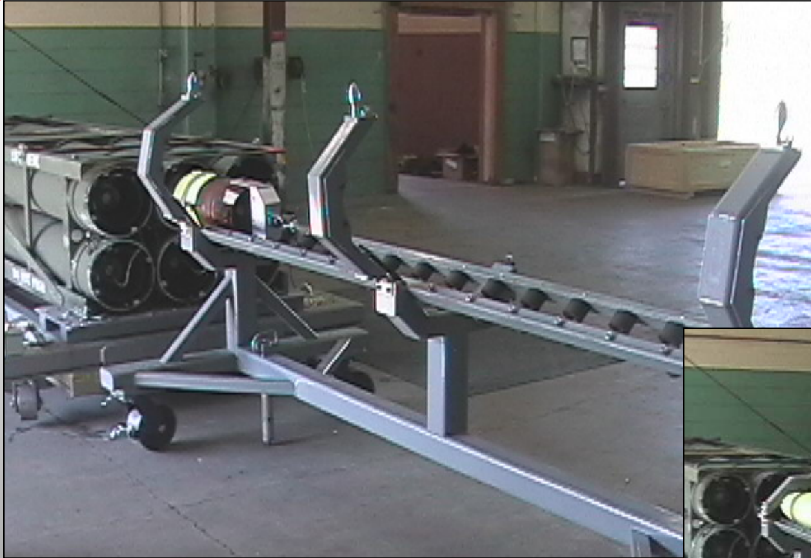
Removal of MLRS Rocket from the Pod
