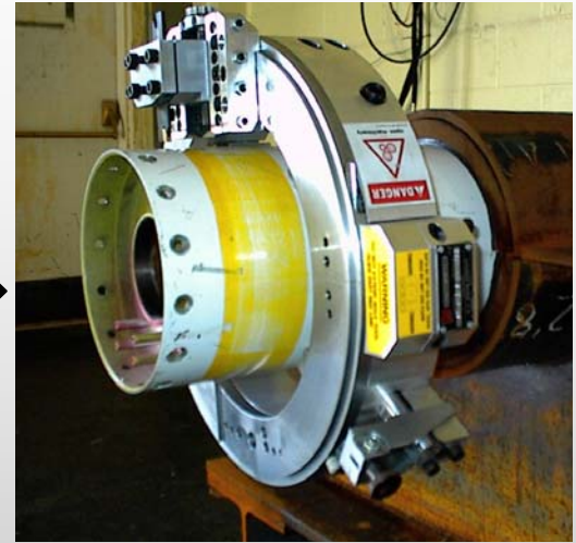
Bulkhead Weldment Removal
