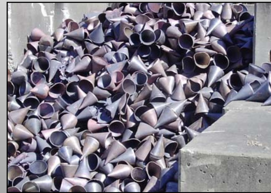
Copper cones after flashing furnace
