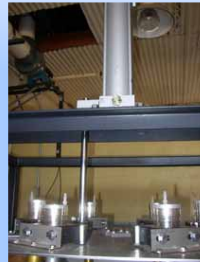
Lift plate holds 6 sonic probe converters.
