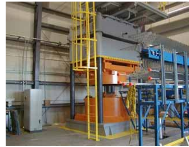
Munitions fractured in press
