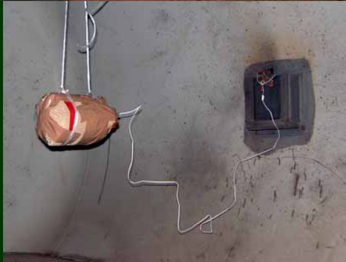
Explosion Experiment Setting, TNT : 2.2kg
