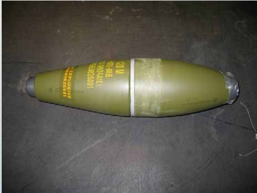
120mm Mortar Prior to Acid Digestion
