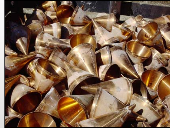
Copper cones prior to flashing furnace
