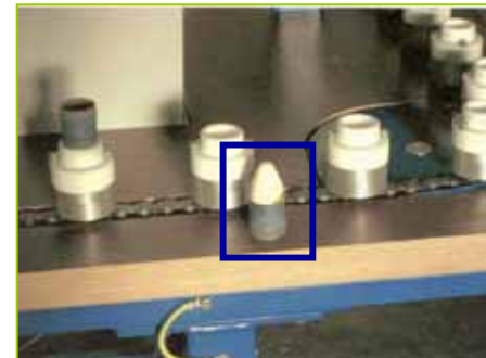
Fuze is Epoxy Locked
