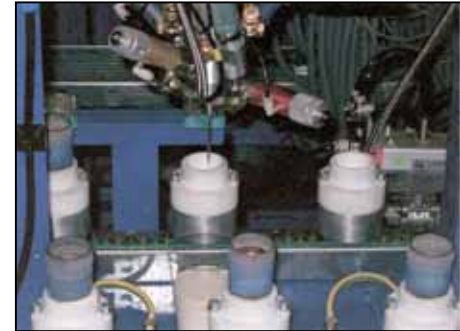
Fuze Mold – Epoxy Fill
