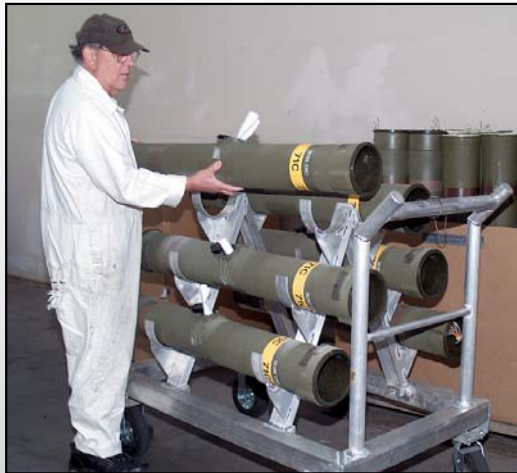
Visual/Physical Inspections Performed on Each Launch Tube
