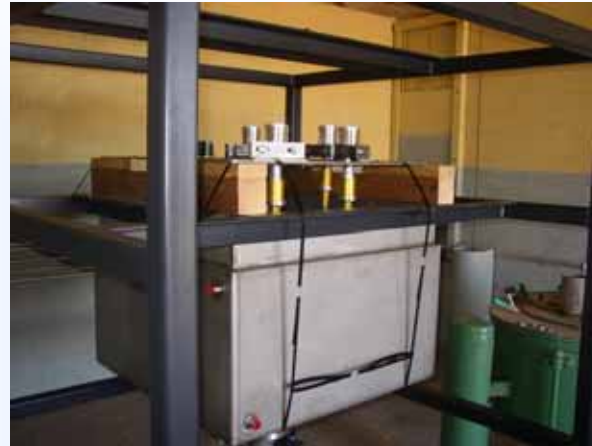
Probes attached to lift plate
