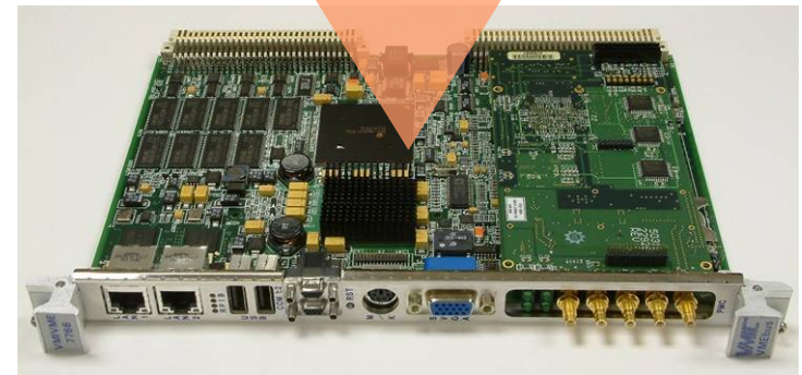
IFD-120 Next Generation SEI Processor mounted on VME Pentium card
