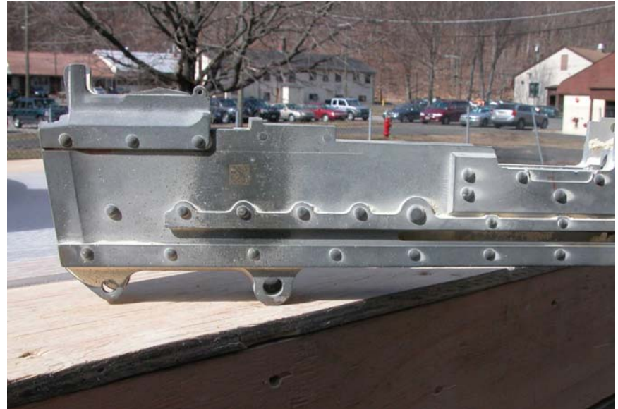
After Sand testing and before cleaning
