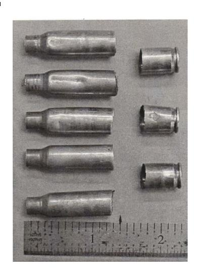
Incidences of the M855 cartridge case rupturing during normal firing of the M249 Saw
