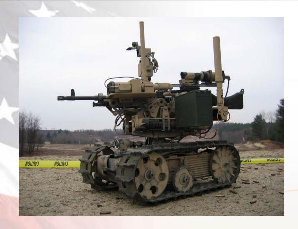
Under partnerships with TACOM-ARDEC and TACOM-TARDEC, Foster-Miller integrated Precision Remote's TRAP system onto the Talon 3B chassis, making the first Special Weapons Observation Remote reconnaissance Direct action System (SWORDS)
