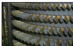
Russian erosion-resistant coating triples life of compressor blades in MH-53 helicopter, avoiding $1.6 million annually
