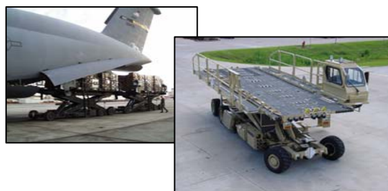
Australian Halverson Loader in use today, replacing unreliable USAF equipment
