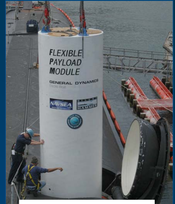
FPM integrated into a missile tube on USS Georgia
