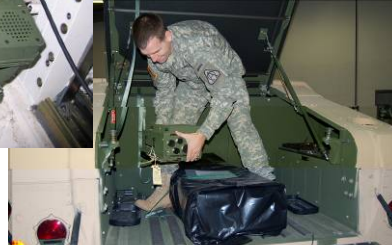
Soldier placing B-Kit Integrated Computer System (ICS) into Current Force HMMWV
