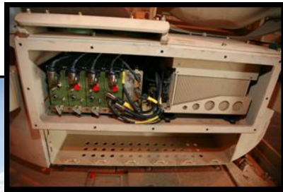
B-Kit components installed into Current Force M1A2 SEP Abrams
