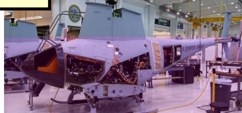
Temporary Nose Cone fitted to Class IV UAV (Fire Scout) A1 preparing for 1st ever Engine Run at Moss Point Facility (May 07)
