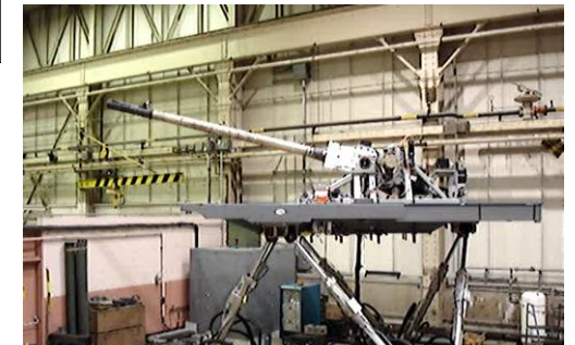
MCS XM360 Electric Gun Elevation Drive Testing
