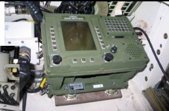
Local Control Display Device installed into Current Force M1A2 SEP Abrams
