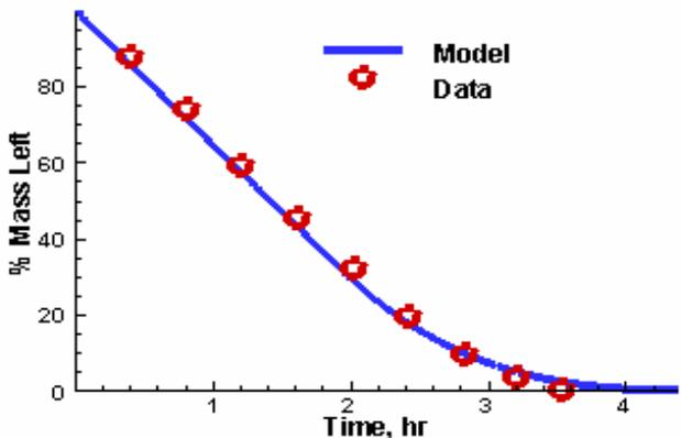
HD on Glass, Wind Velocity = 1.77 m/s, Drop Size = 6  $\mu$ L
