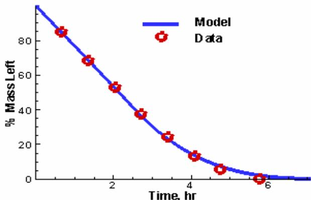
HD on Glass, Wind Velocity = 3.66 m/s, Drop Size = 1  $\mu$ L
