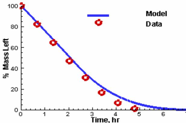
HD on Glass, Wind Velocity = 1.77 m/s, Drop Size = 6  $\mu$ L
