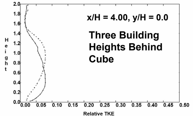
H is building height,  $x/H=0.0$  is upwind face of building and  $x/H=1.0$  is downwind face of building, U is wind velocity,  $U_b$  is mean wind velocity and TKE is Turbulent Kinetic Energy.
