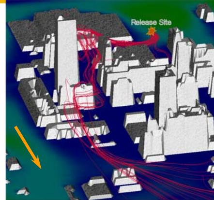
Streamlines Predicted by RUSTIC in OK City. Turbulence Produces Complex and Non-intuitive Flow (above).
