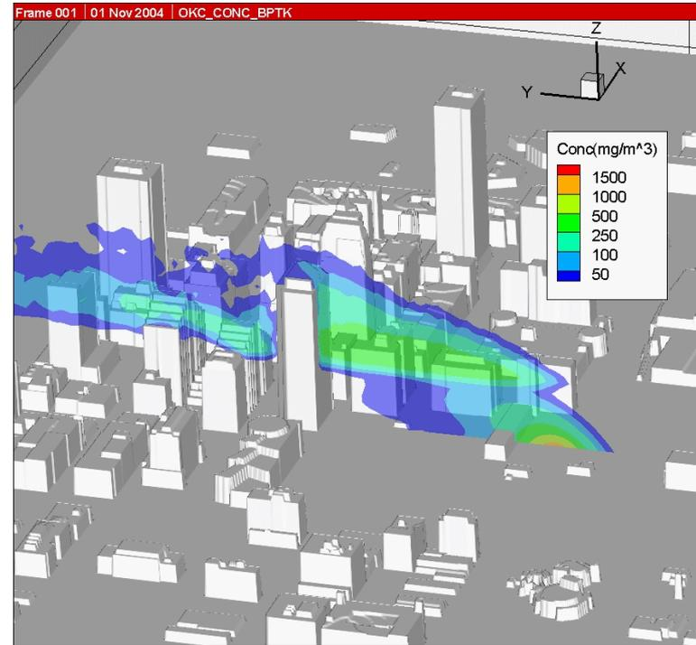
Simulated concentration levels for volatile drops release in Oklahoma City
