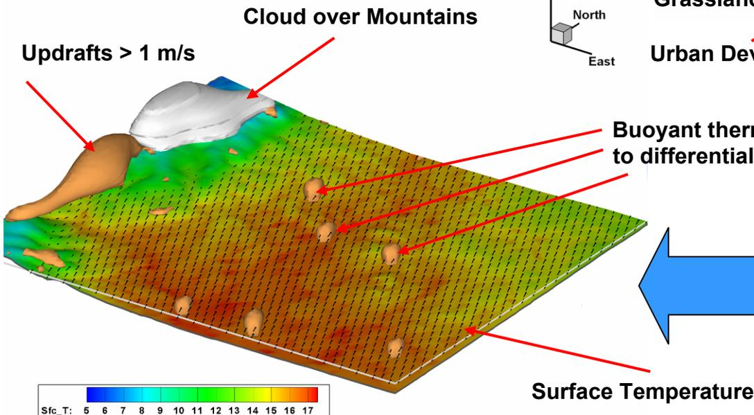
Simulation for Colorado Springs area with winds from  $160^\circ$  on a 20 km x 20 km grid
