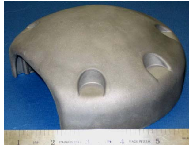
Actuator Mount Cap for the EFV cast using Metal Mold
