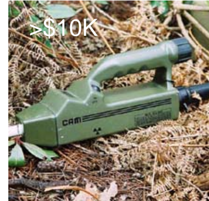
CAM: ion mobility spectrometry
