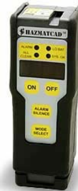
HAZMATCAD: electronic nose using SAWs and ECs
